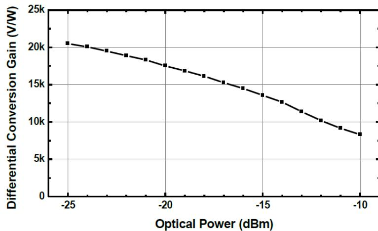
Differential conversion gain over 20000 V/W, roughly matches the device datasheet:
