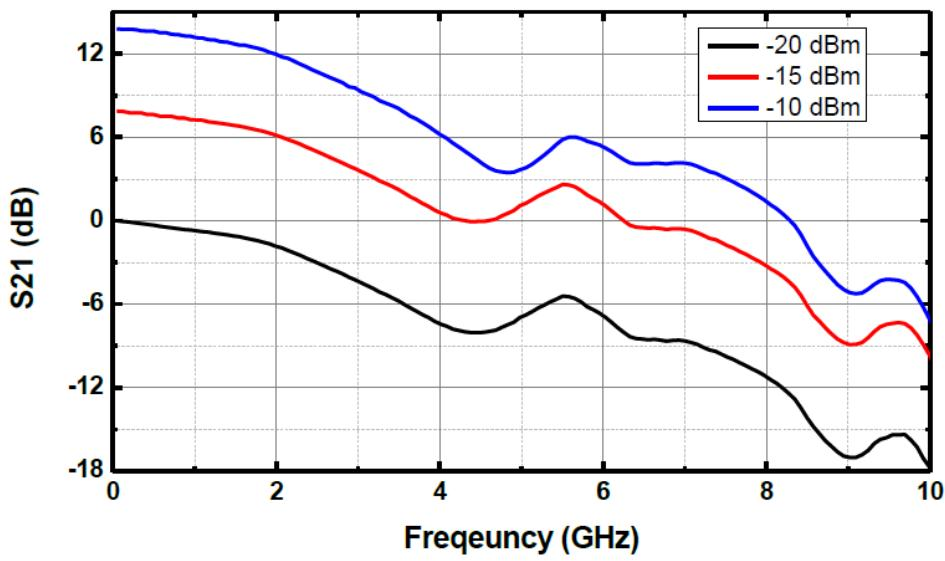
S21 curve at three different optical input power level: -20 / -15 / -10 dBm
